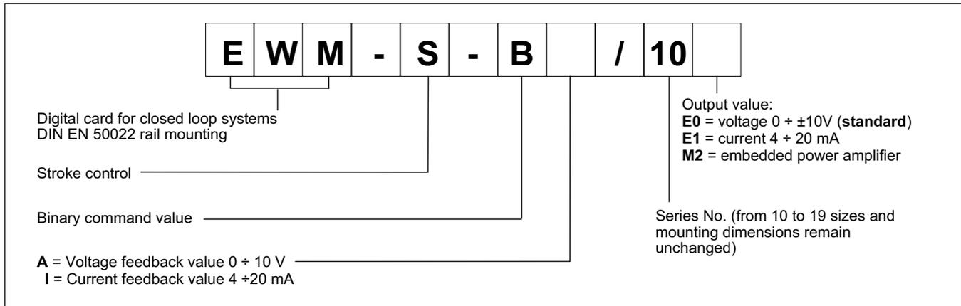
This module supports the simple point-to-point positioning with hydraulic drives. Two operating modes can be selected: stroke depending deceleration, that means the control gain will be adjusted with the parameters D:A and D:B, and NC mode, where the position value is generated from the following error.
